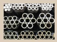
(CC 493K) is a tin bronze product and one of the most commonly available bronze alloys due to the materials excellent allround capabilities. Offering good dry running characteristics and pressuretightness, RG7 is easy to machine and finds use in the production of slide bearings and bearing bushings.
