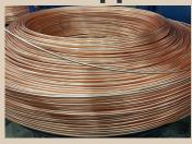
Oxygen-free copper (OFC) copper is a group of wrought high-conductivity copper alloys that have been electrolytically refined to reduce the level of oxygen to 0.001% or below.
