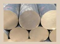
Red brass has an excellent resistance to dezincification and season cracking. Red brass is commonly specified for underground service lines, and it offers the greatest corrosion resistance when used in potable water applications
