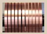
C14700 is a high conductivity copper with added sulphur to provide free-machining characteristics. Sulphur bearing copper has excellent machinability.
