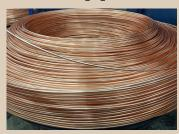
Electrolytic-Tough-Pitch (ETP) is the most common copper alloy. It is used universally for electrical applications due to its minimum conductivity and 100% IACS (International Annealed Copper Standard) rating.
