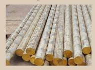
Binary Brass is a series of binary alloys between copper and zinc, with an upper zinc content of about 40%.
