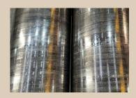
The B14 alloy is a very hard, tough bronze with good sliding properties and excellent corrosion resistance. Withstands great efforts, impacts, wear, abrasion, fatigue and high temperature; resistant to high hydraulic pressures, good anti-friction quality.
