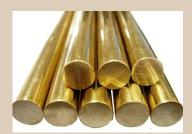
Cartridge Brass, also known as 70/30, is copper alloyed with zinc. C260 is a yellow brass with fair to excellent corrosion resistance. Excellent cold workability and good hot formability.
