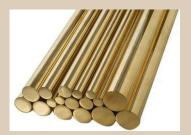
This product is sometimes referred to as Arsenical Brass. It is copper alloyed with tin and zinc. Brass C443 has good corrosion resistance and excellent heat transfer characteristics. This type of brass has found use in fresh, brackish and saltwater applications, as well as oil and gas systems where there are corrosive resistant tubes.
